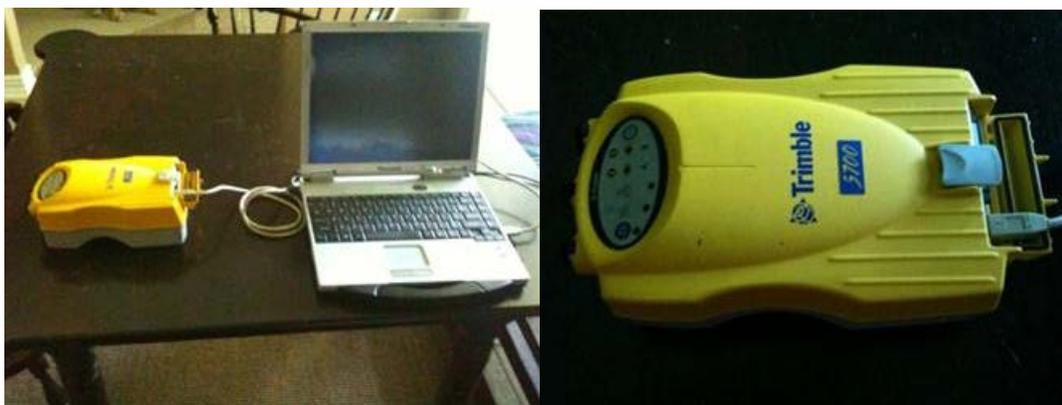
1. Turn on 5700 by pressing and holding the green power button on the receiver control panel until the indicator lights come on.
