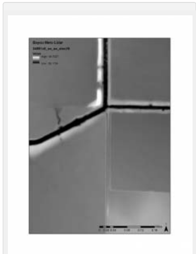
Bare earth DTM created before manual re-classification.
