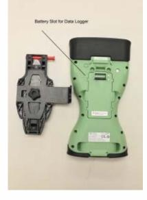
You can hot-swap one of the two batteries. In operation battery status on GPS is shown via "Power LEDs". One battery will be "active" one "passive"
