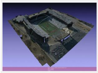
3D model of Razorback Stadium created from four digital aerial images using PhotoScan Pro (model shown here in Meshlab software)
