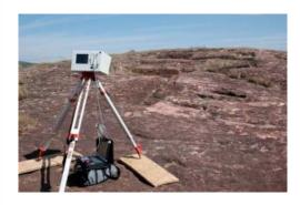
3D scanners allow for a large number of measurements to be collected across the surface of a structure, landscape or object, resulting in a dense three-dimensional digital data file that accurately portrays surface features. The data collected are an accurate mapping of the surface which cannot be obtained as easily or as accurately by traditional surveying or other recording
