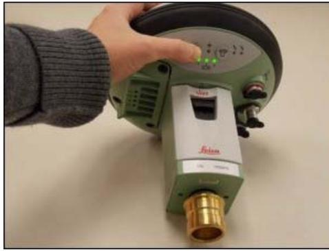
Note: It is important to understand what the buttons, symbols, and LED lights do and/or represent on the GS15 unit. A detailed description of button operation can be found in the Leica "GS10/GS15 User Manual" in section 2.1, pages 20-24. A detailed description of symbols and LEDs can be found in the same manual in section 3.5, pages 64-68. The GS15 is powered down by pressing and holding the power button until the LEDs turn red.
