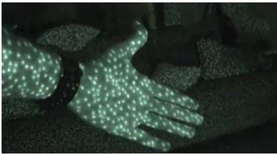
The popular hardware stack that is known world-wide as the "Kinect" is very different from the rest of the scanners owned by CAST. Essentially, it is a low cost stack of hardware sensors used to capture comparatively low resolution 3D data. The Kinect has applications in academia, and is employed across a wide variety of fields for research tasks requiring the ability to track motion, detect change, and produce 3D models of a manageable size.
