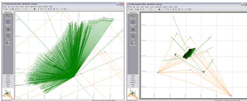
Green vectors represent measures from the 5600 total station to an active prism pole as part of a micro-topography survey. The orange vectors represent GPS base-lines measured in fast-static mode using the 5700/5800 instruments. The GPS observations were integrated with the total station survey to establish a geodetic reference for the survey.
