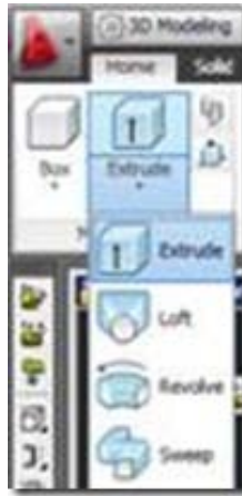
Figure 4 Extrude icon pulls down to reveal Loft and Revolve Icons in the 3D Modeling Workspace or enter LOFT at command line
