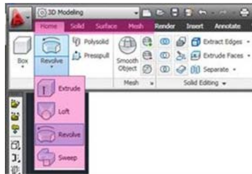
Figure 1 – Main ACAD toolbar with modeling tabs highlighted in Magenta; EXTRUDE, LOFT, REVOLVE, AND SWEEP exist on each of the modeling tabs. Which tab is active and whether the polyline is open or closed determines what type of object is created.
