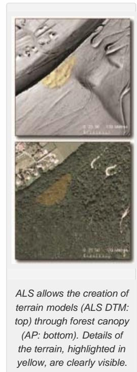
ALS allows the creation of terrain models (ALS DTM: top) through forest canopy (AP: bottom). Details of the terrain, highlighted in yellow, are clearly visible.
