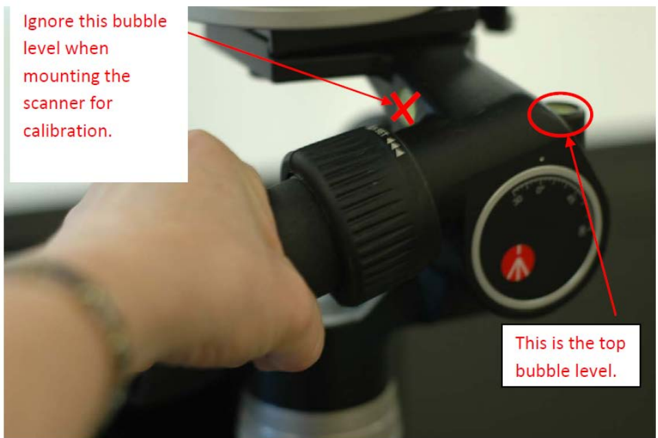
Fig. 8: The top bubble level.
