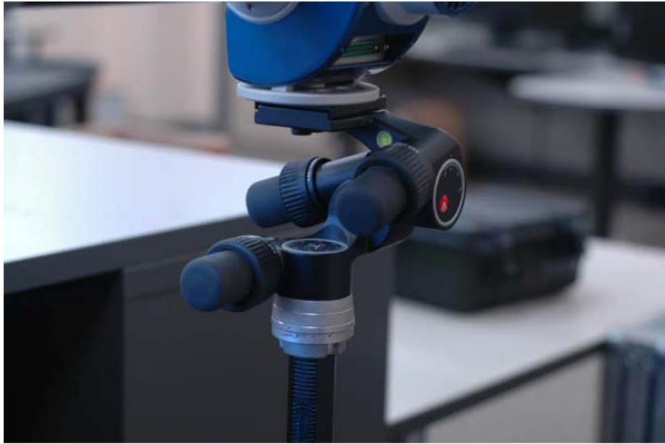
Fig. 11: The scanner mounted on the level tripod.
