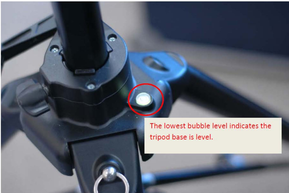
Fig.3: The lowest bubble level
