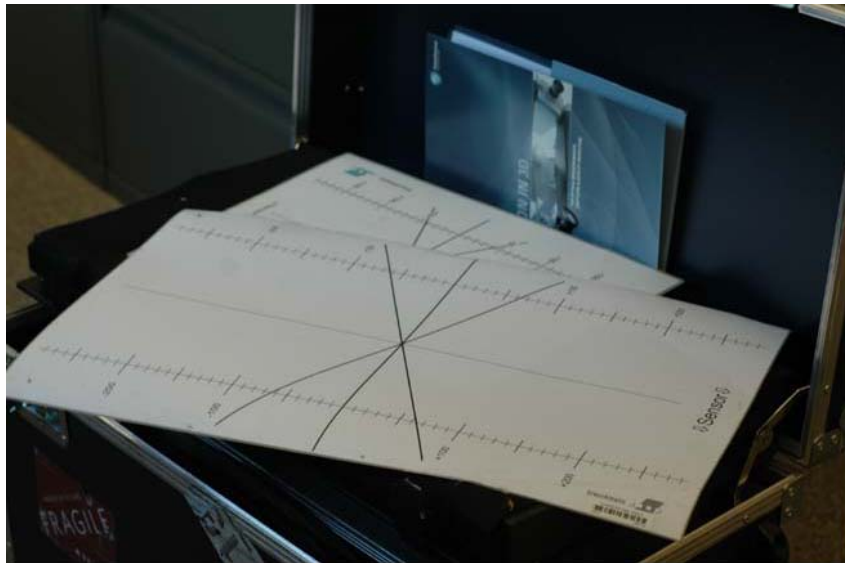
Fig.12: The datasheet and chart placement guide in the scanner case.
