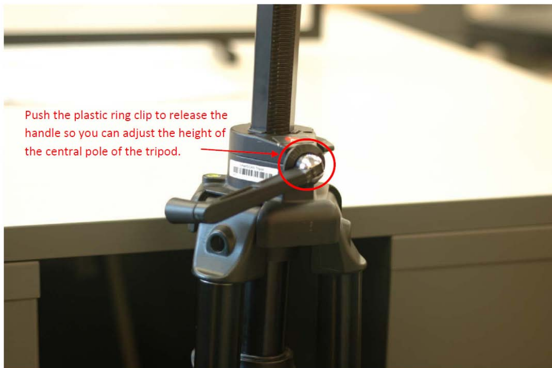
Fig.5: The central pole height is adjusted by turning this handle.
