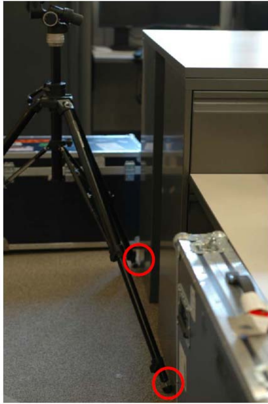
Fig.2: Tripod feet are level and flush with the base of the desk
