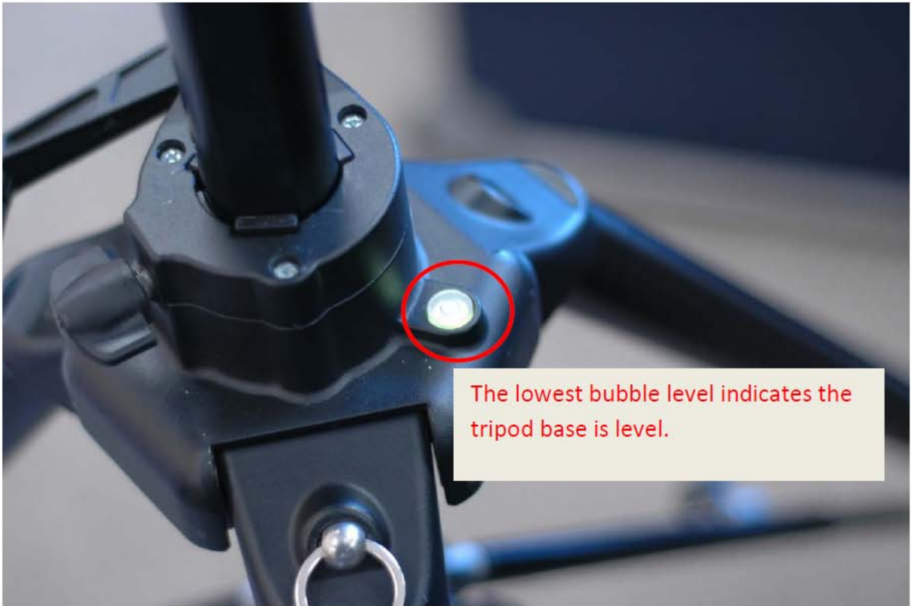
Fig.3: The lowest bubble level
