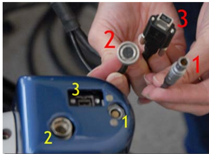
Figure 8: Three camera cables and their associated connections
