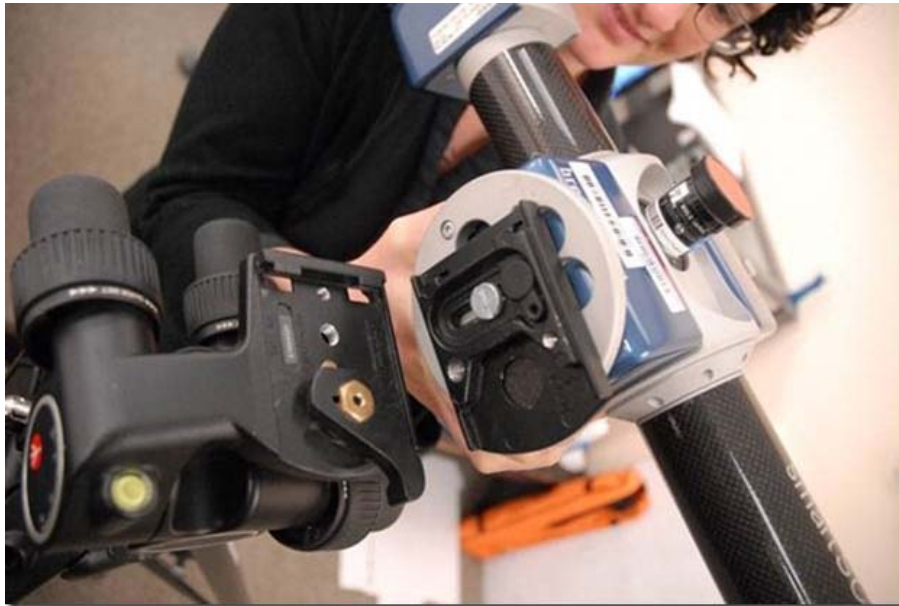
Figure 4: Placing the scanner onto the tripod
