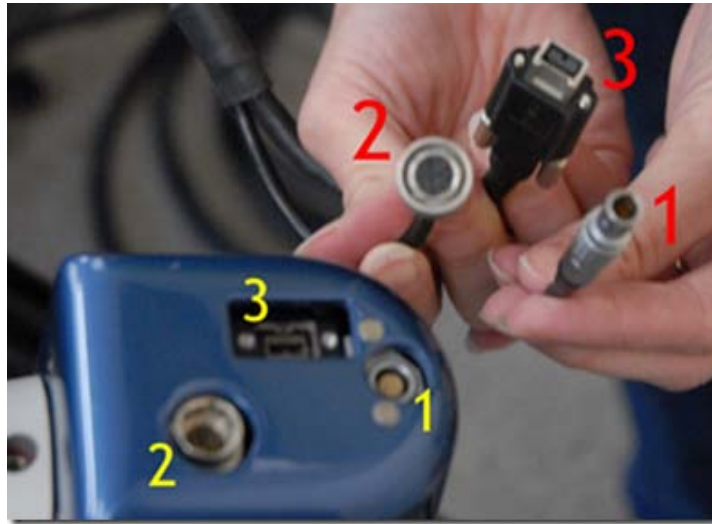
Figure 12: Image showing three cables/connections for each camera
