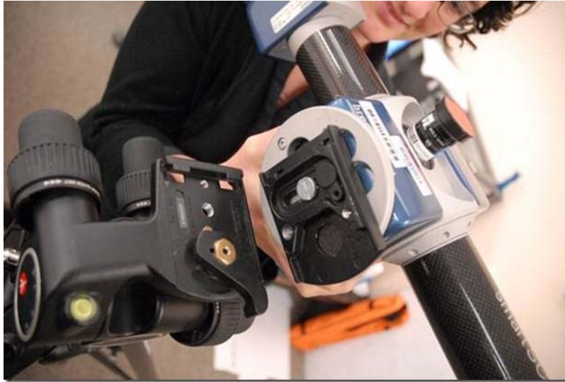
Figure 4: Placing the scanner onto the tripod
