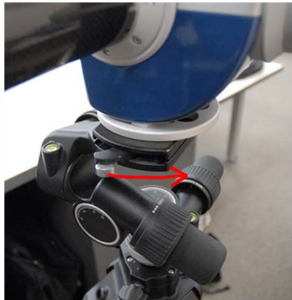
Figure 13: Pull silver lever towards the back of the scanner to remove the scanner from the tripod
