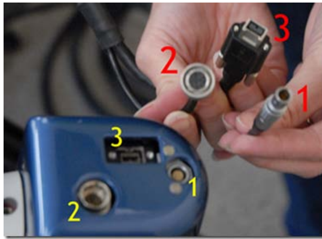
Figure 8: Three camera cables and their associated connections
