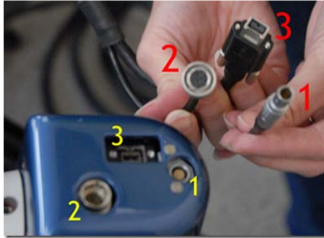
Figure 12: Image showing three cables/connections for each camera
