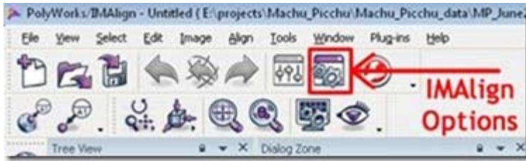
Figure 7: Remember to set IMAlign options as suggested below prior to importing any data
