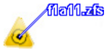
Figure 1 – Hyperlink that allows you to enter viewpoint of the scanner position from the TruView site map. The number represents the scanner station identification.
