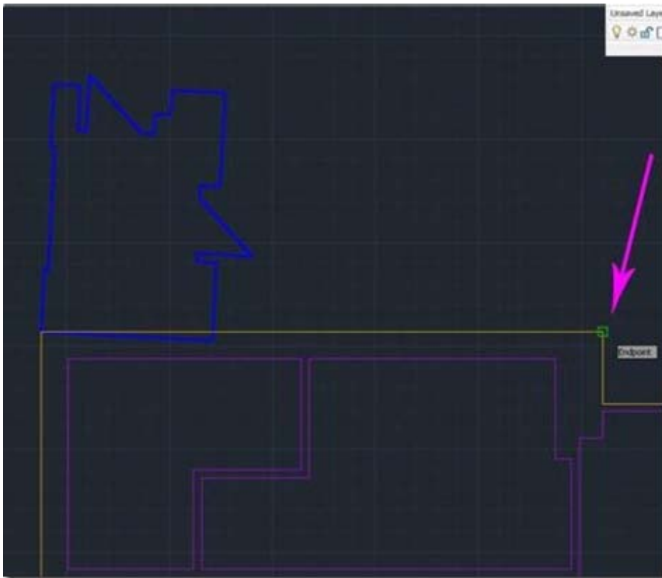
Figure 6 – A significant point on the block object is selected for the 2nd source point – here, another corner is used
