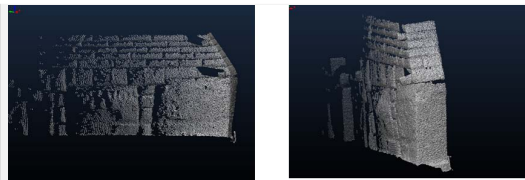
Left shows a stone wall scanned from a perpendicular angle; points are gridded evenly across the surface. Right shows the same wall scanned with a high angle of incidence. The density of the points changes as the distance and angle increases.
