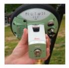
Stand the fixed-height tripod on its center tip, loosen the brass thumbscrew in the side of the top mounting plate, insert the brass adapter on the antenna into the mounting hole, and then tighten the thumbscrew.
