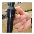
Loosen this thumbscrew, and then extend the leg and place its tip as you did on the other two legs. Be sure to leave the thumbscrew <u>loose</u>. At this time, if your are on soft ground, you should use your foot to push each of the three legs (not the center pole) into the ground.
