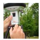
At the base of the tripod, flip the lever to release the center leg, and then extend it fully to the 2-meter mark.
