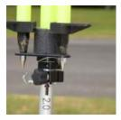
Carefully place the tip of the center pole at the exact spot on the ground that you wish to survey.
