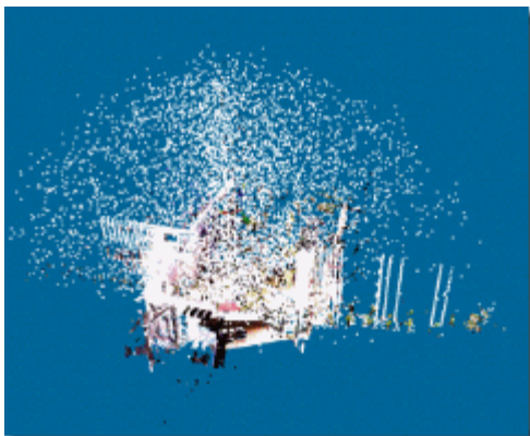
Figure 4: Extraneous data in the scan that will need to be filtered out
