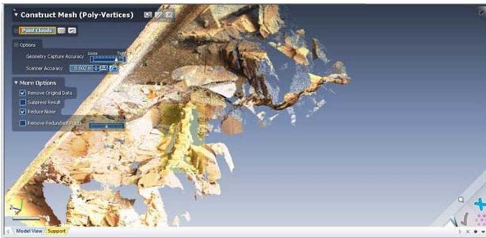
Fig. 15: Limited area mesh construction.
