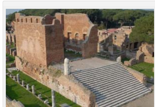
"Good" close-range photogrammetry example from Ostia Antica, Italy. Note that the object (the temple) is framed tightly, and that all objects (both near and far) are in sharp focus.
