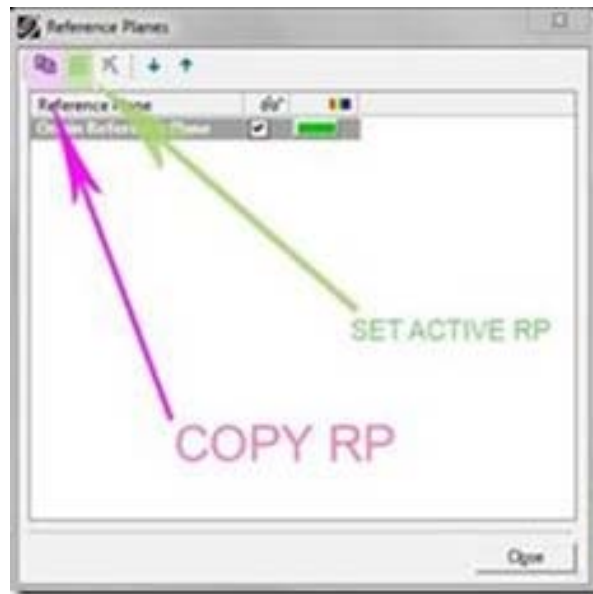
Figure 2 (Left) – A closer view of the dialog box and the options for copying/adding RP’s and for activating the RP
