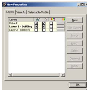
Figure 1: Use the Shift+L button to open the Layers Dialog. Here you can create new layers, set the current layer, and select and assign objects to layers.
