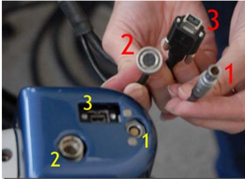
Figure 8: Three camera cables and their associated connections
