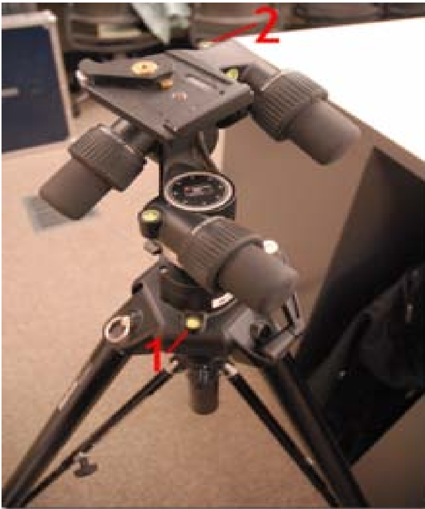
Figure 2: Tripod levels. Only use levels 1 and 2 when leveling the tripod.
