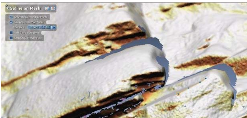
Fig. 32: Drawing a spline on a mesh.
