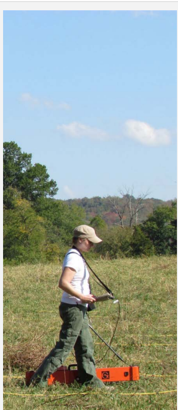
Stephanie Sullivan using a Geonics EM38-MK2 Conductivity Meter
