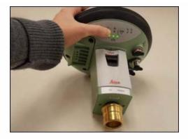
Note: It is important to understand what the buttons, symbols, and LED lights do and/or represent on the GS15 unit. A detailed description of button operation can be found in the Leica "GS10/GS15 User Manual" in section 2.1, pages 20-24. A detailed description of symbols and LEDs can be found in the same manual in section 3.5, pages 64-68. The GS15 is powered down by pressing and holding the power button until the LEDs turn red.
