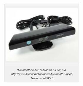
The Kinect camera is an RGB device with a resolution of 640×480 and a 24 bit color range (Red- Green- Blue channels).
