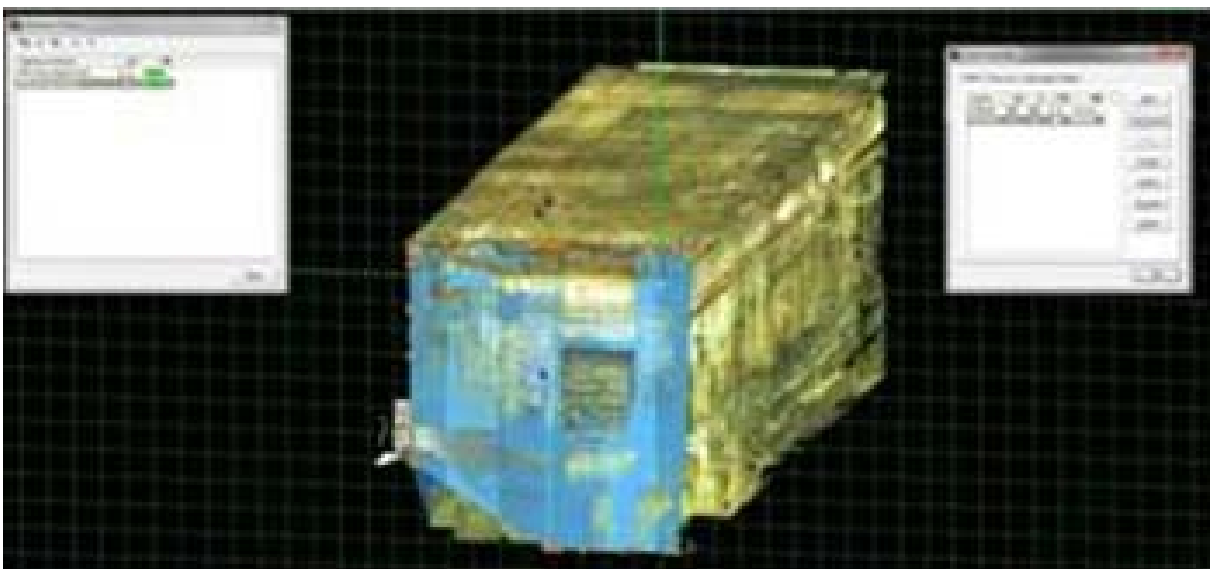
Figure 9 “ The vertical reference plane is aligned to the wall/patch
