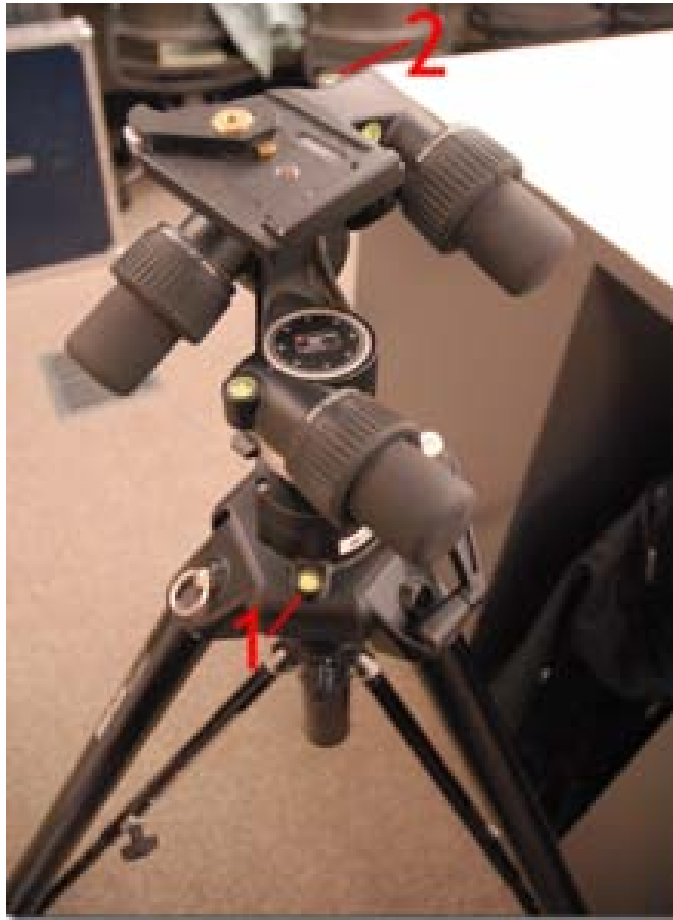
Figure 2: Tripod levels. Only use levels 1 and 2 when leveling the tripod.
