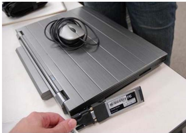
Figure 11: Express card adapter that fits the Express card slot on the laptop
