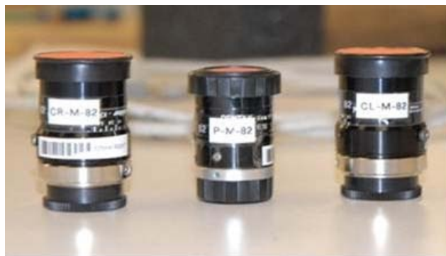
Figure 5: Set of lenses for the 825mm FOV (CR = Camera Right, P=Projector, and CL = Camera Left)
