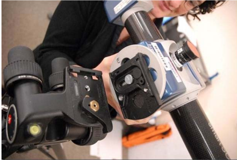
Figure 4: Placing the scanner onto the tripod
