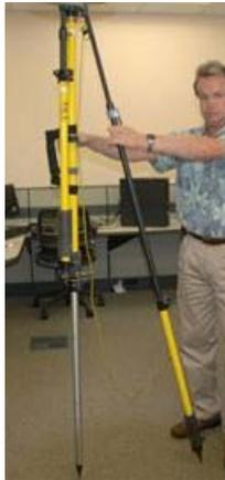
9. The third leg is different; instead of a squeeze clamp, it uses a thumb screw to tighten the upper section. Loosen this thumbscrew, and then extend the leg and place its tip as you did on the other two legs. Be sure to leave the thumbscrew loose. At this time, if you are on soft ground, you should use your foot to push each of the three legs (not the center pole) into the ground.
