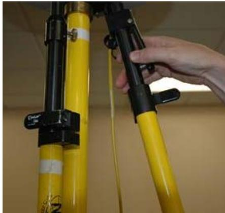
Angle the leg away from the tripod body and flip the lever to release the lower clamp on the leg. Extend the lower portion of the leg all the way, and then lock the clamp again.
