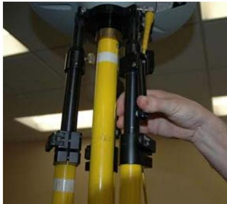
To release them from the tripod base, squeeze the clamp and lift the leg up so that the tip clears the base.
