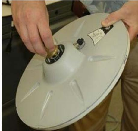
2. Stand the fixed-height tripod on its center tip, loosen the brass thumbscrew in the side of the top mounting plate, insert the brass adapter on the Zephyr antenna into the mounting hole, and then tighten the thumbscrew.
