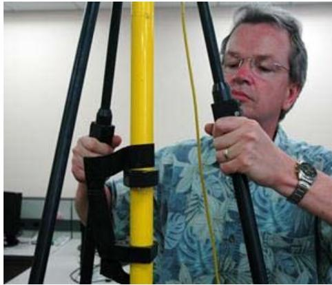
11. If the field case for the receiver you're using has cable pass-through (a black, round plug in the side of the case), you can unscrew it and thread the antenna cable through the opening (this will let you put the receiver and batteries in the case with the lid shut). Regardless of which case you're using, the next step is to remove the cap for the antenna connector on the 5700 receiver, and then connect the yellow antenna cable.
