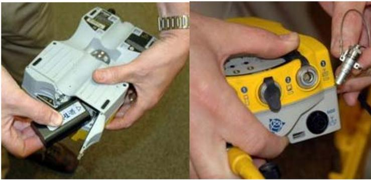
13. When disconnecting the battery pack, release the plug by pulling on the steel wire loop attached to it.
