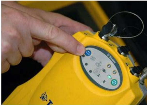
The red SV Tracking LED below the satellite icon indicates the status of satellite tracking:
