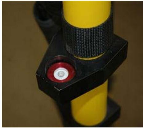
Place a hand on each of the squeeze clamps, squeeze them to release their lock, and very carefully push or pull to align the air bubble in the level within the inner marked circle. When you have the tripod level, release both of the squeeze clamps, and check your level again. If it is still level, lock the thumbscrew on the third leg, and you are finished with the tripod.
