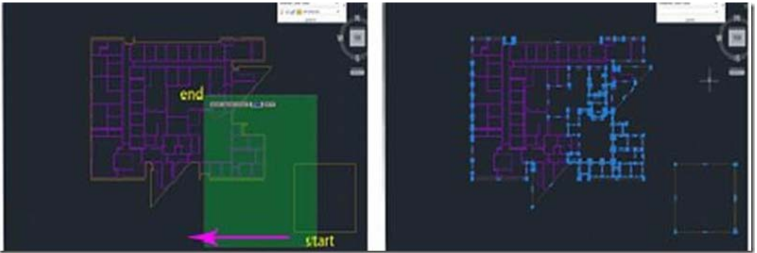
Figure 6 – (Left) Selection Window drawn right-to-left with start and end points marked. (Right) The grips (blue "dots") of all objects selected are highlighted – Again, note the yellow rectangle in the lower right hand of the screen; the selection window touched the box, therefore it is selected
