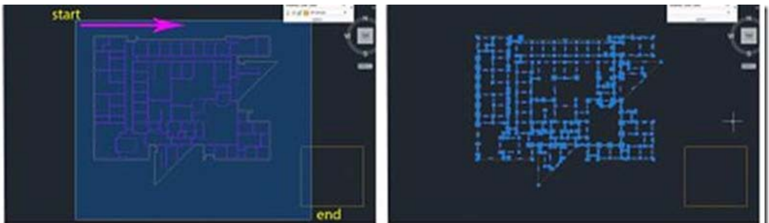
Figure 5 – (Left) Selection Window drawn left-to-right with start and end points marked. (Right) The grips (blue "dots") of all objects selected are highlighted – Note the yellow rectangle in the lower right hand of the screen; although the selection window touched the rectangle, it did not enclose it, therefore it is not selected
