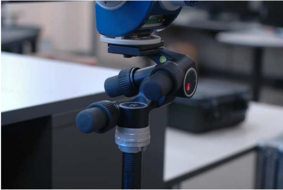
Fig. 11: The scanner mounted on the level tripod.
