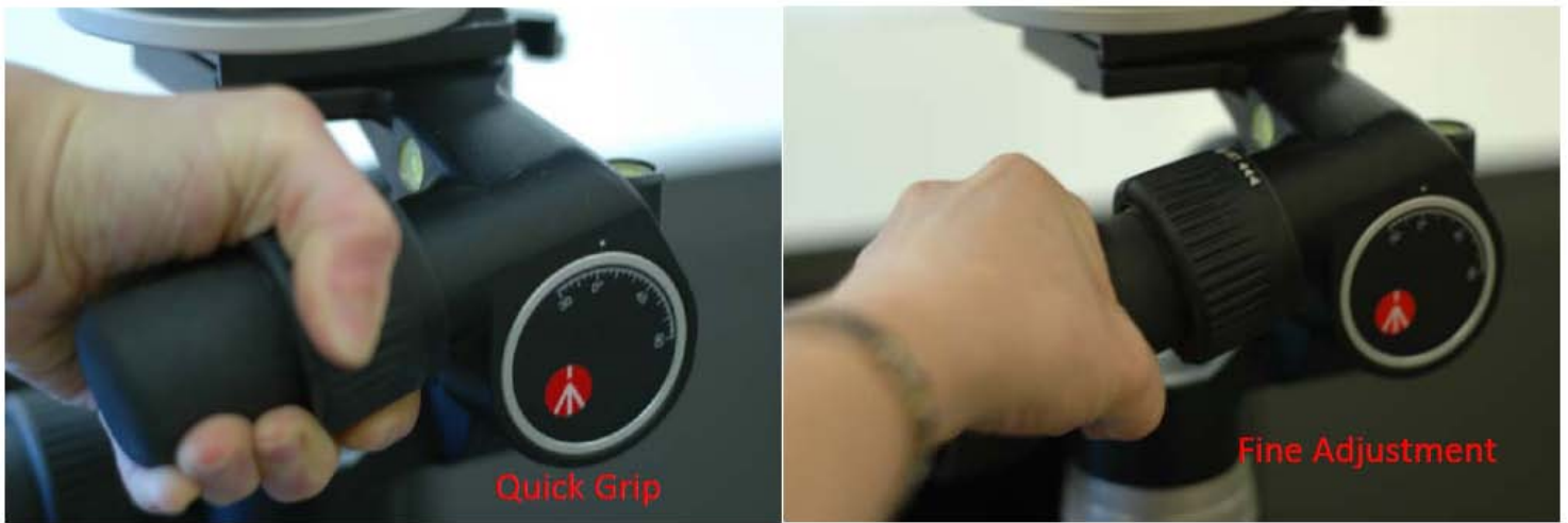
Fig.10: Quick grip and fine adjustment positions on the adjustment handles of the tripod head.
